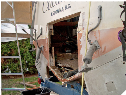
TOP: The rot got worse towards the sides of the hull.
